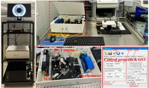
**Figure 2.** Photos of portable OCT system operating at 800 nm, the OCT engine, the control program and its GUI. Based on the first benchtop system, we have further developed <u>a portable 800-nm ultrahigh resolution OCT</u> system based on spectral-domain OCT (SD-OCT) configuration. With this rotary joint the imaging speed can be
