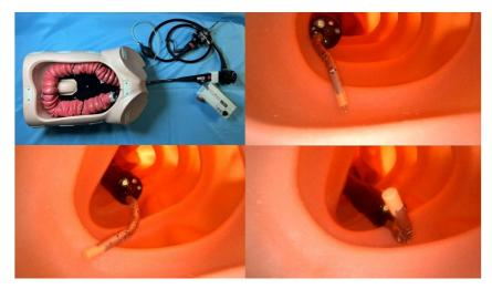
Fig. 7. Demonstration of manipulating the hand-held steerable endoscopic robot in a phantom colon.
