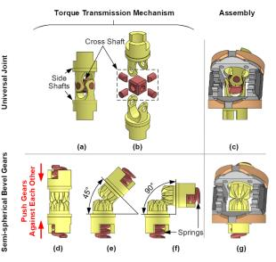
Figure 14 Torque transmission mechanisms. (a) Universal joint assembly; (b)exploded view of (a); (c) joint assembly with a universal joint  $(\theta=30^\circ)$ ;(d)-(f) semi-spherical bevel gears when joint angle  $\theta=0^\circ$ , 45°, and 90°, respectively; (g) joint assembly with semi-spherical bevel gears.
