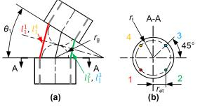
Figure 19 (a) Geometry of Joint 1 of the drilling wrist; (b) Cross-section view for tendon location.
