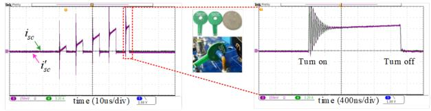
Fig. 1. Illustration of measured current following actual current accurately (actual current measured with Tektronix TCP0030A current probe with a bandwidth of 120MHz).
