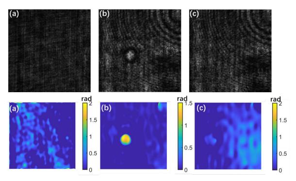
Fig. 7. Validation of using phase conjugation for cancellation the phase of a 5  $\mu$  m bead. (a) Background interferogram without sample; (b) interferogram with the sample moved to the field of view; (c) interferogram after conducting the phase conjugation experiment. (d), (e), and (f) correspond to the retrieved phase maps of (a), (b), and (c), respectively.
