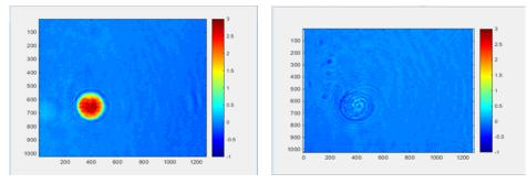
Fig. 2. Cancellation of the phase of a 10  $\mu m$  bead.
