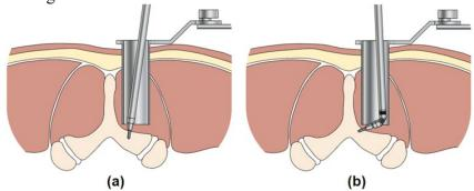
Figure 12 Conceptual view of drills in minimally invasive spine surgery. (a)Conventional straight-shaft drill; (b) articulated steerable drill.
