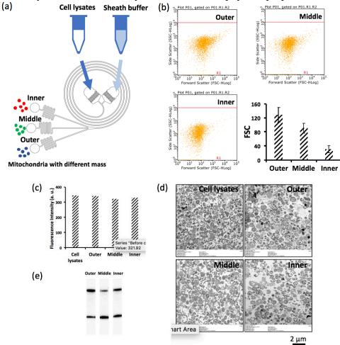
Figure 3. (a) Overview of the chip. (b) Scatter plot of mitochondria subpopulations analysed by flow cytometer. Intactness of mitochondria validated by (c) mitotracker staining and (d) TEM. (e) Mitochondrial functionalities measured by DNA repair assay.
