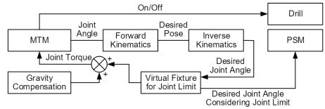
Figure 21 Control scheme of the proposed drilling system.
