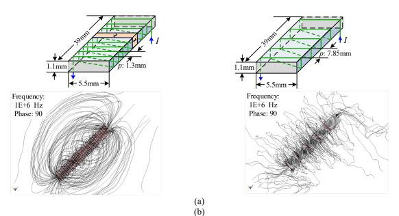
Fig. 2. Structures and longitudinal magnetic field distributions of (a) thirty-turn and (b) five-turn PCB coils.
