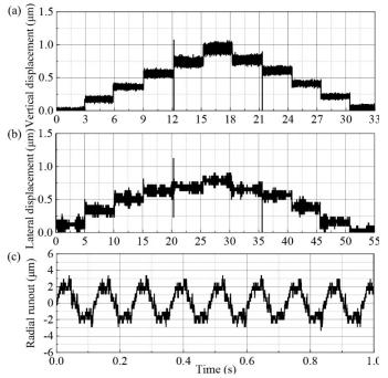
Figure 5. Active axis position control in the (a) vertical and (b) lateral directions; and (c) shaft runout during rotation.
