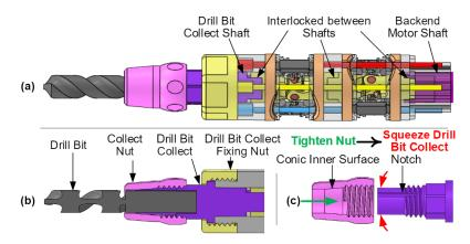
Figure 15 Drill tip assembly. (a) Torque transmission between shafts; (b) Cross section view of drill bit and its holder; (c) drill bit holding principle.
