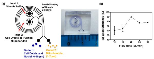
Figure 1. (a) Schematic showing the design of the chip. (b) Optimization of flow rates using purified mitochondria.
