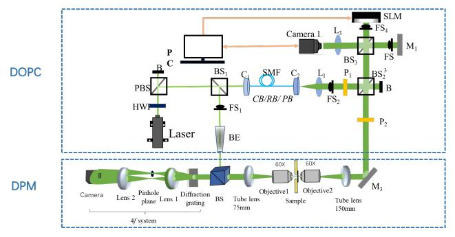
Fig. 5. The integrated system that contains digital optical phase conjugation (DOPC) and DPM.
