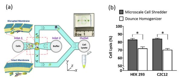
Figure 4: (a) Schematic illustrations of the concept of cell lysis using hydrodynamic shear stress. (b) Comparison of cell lysis efficiency between the on-chip shearing and the Dounce Homogenizer. Results were plotted as mean  $\pm$  S.D. (n = 3 independent experiments, \*P <0.05).
