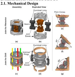
Figure 13 Design of a tendon-driven rolling joint with an inner lumen. (a)Joint assembly for the retractor; (b) exploded view of (a);
