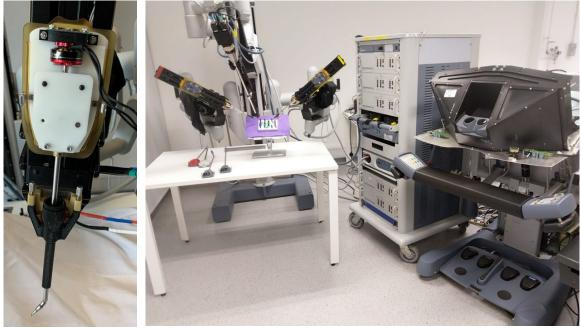
Figure 18 Proposed drilling instrument integrated with the dVRK.
