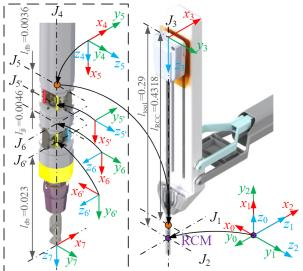
Figure 20 Frame definition of the proposed drilling system (unit: meter).
