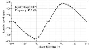
Figure 3. The relationship between rotation speed and phase angle.
