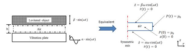
Figure 7. Schematics of forced vibration system (left) and equivalent model of the system (right)
