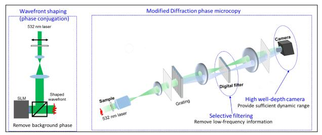
Fig. 1. Proposed design of the highly sensitive QPM system.
