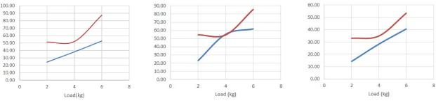
Fig. 6. Summary of human experiments. Load vs EMG reading without robot (red) and with robot (blue). Anterior for flexion motion (left), middle for abduction (middle) and posterior for extension (right).
