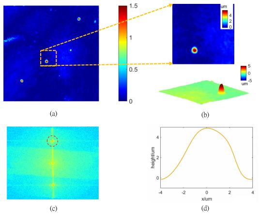
Fig. 4. DPM system validation. (a) Phase map of a captured interferogram; (b) a zoom-in height map of (a); (c) the Fourier spectrum modulus of the interferogram; (d) a line profile of the  $5 \mu$  m bead.
