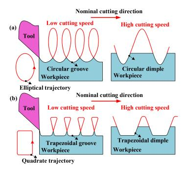
Fig. 10. Comparison of elliptical vibration texturing and quadrate vibration texturing.
