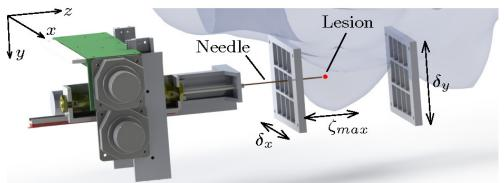
Figure 2 Details of the needle driving mechanism
