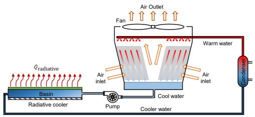
Figure 1. Schematic of the proposed cooling tower with renewable passive radiative cooling.
