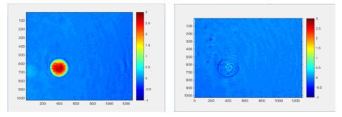
Fig. 2. Cancellation of the phase of a 10 µm bead.
