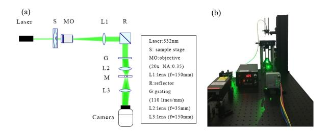
Fig. 3. (a) Schematic design of the QPM system; (b) the photo of the actual QPM system.
