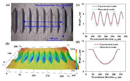
Fig. 9 (a) Measured topography of the machined texture, (b) 3D topography, (c) sectional profile of xmdirection from the measured topography, (d) sectional profile of ym- direction from the measured topography
