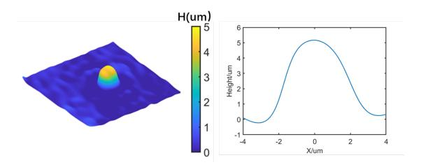
Fig. 6. The height map and line profile images of the 5um beads.
