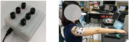
Fig. 4. Command mode of robot: 1) potentiometers dials for each muscle (left); 2) EMG on muscles (right)
