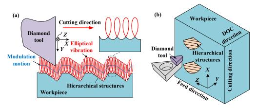
Fig. 4 Principle of hierarchical structures fabrication.
