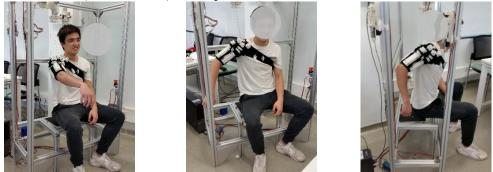
*Fig. 2. Flexion (left), abduction (middle) and extension (right) motions of the shoulder produced through the robot prototype using the Myomuscle actuator units*
