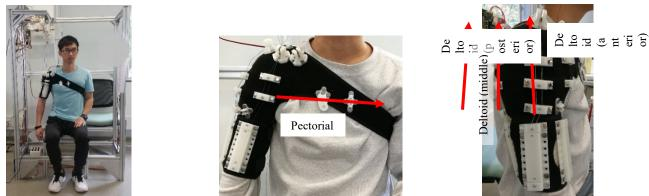
Fig. 1. Exo-muscular robot prototype. Overall view (left), front view (middle) and side view (right).
