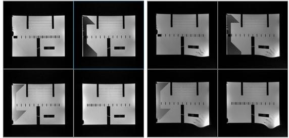
Figure 8 MRI scans to compare the compatibility of our actuator. (left) Scan with the Tesla motor, and (right) scan with a commercial piezo-electric motor.
