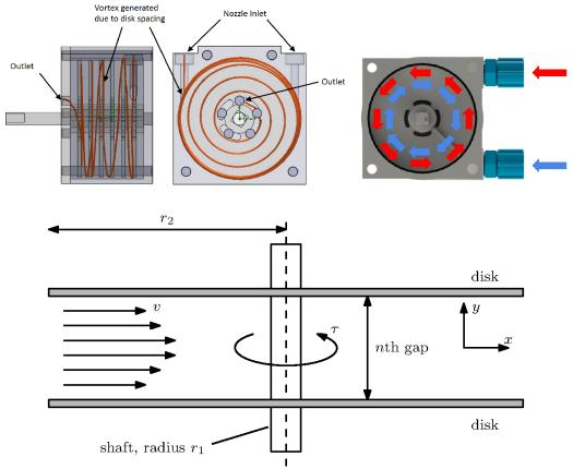
Figure 5 Working principle of the pneumatic actuator
