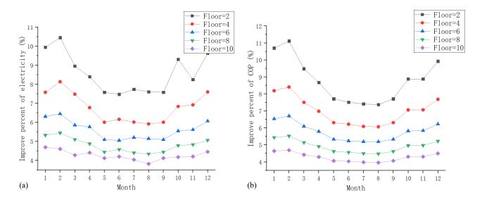
Figure 3. (a) Percentage of reduction in chiller electricity use, and (b) percentage of increase in chiller COP.
