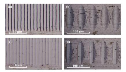
Fig. 11. Topography of textured sruface with the elliptical trajeocty at 300 Hz: (a) cutting speed of 0.6 mm/s and (b) cutting speed of 15 mm/s; with the quadrate trajectory at 300 Hz: (c) cutting speed of 0.6 mm/s and (d) cutting speed of 15 mm/s.
