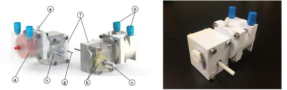
Figure 6 (Left) Schematic drawing of Tesla motor: (a) disks assembly, (b) worm gears, (c) output shaft, (d) inlets ports, (e) silencer, (f) optical fibre, (g) rotary encoder (h) encoder disc. (Right) Prototype of Tesla motor
