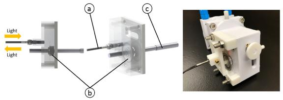
Figure 7 (Left) Details of the proposed rotary encoder, where: (a) optical fibre; (b) encoder disk; (c) output shaft. (Right) The developed prototype for the MRI-compatible sensor.
