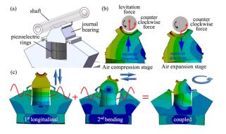
Figure 1. (a) Design of a single driving unit; (b) operation principle for shaft levitation and rotation; and (c) coupled mode shapes.
