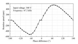
Figure 2. The relationship between rotation speed and phase angle.
