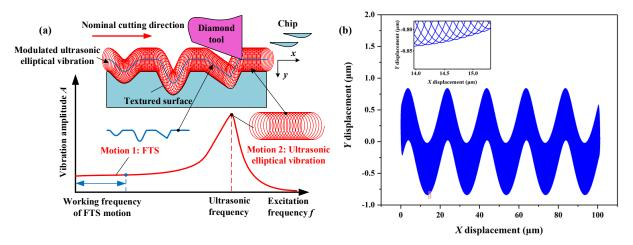
Fig. 7 (a) Principle of surface texturing of silicon, (b) tool moving trajectory, (c) machined dimple patterns
