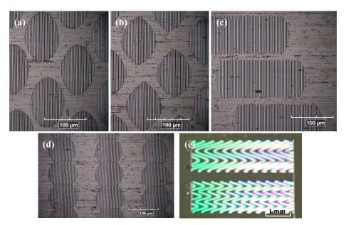
Fig. 6 machined hierarchical dimples and grooves. (a) circular dimple (b) triangle dimple (c) trapezoidal dimple (e) straight groove (e) bending groove
