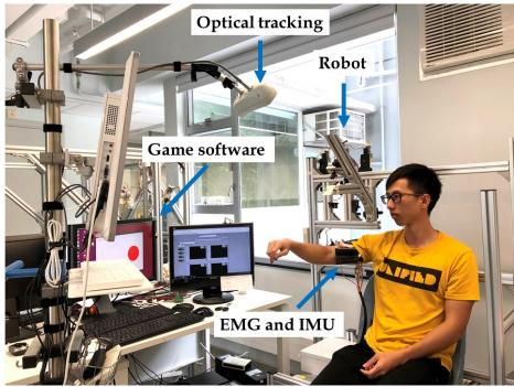
Fig. 3. Complete musculoskeletal robot rehabilitation and exercise system
