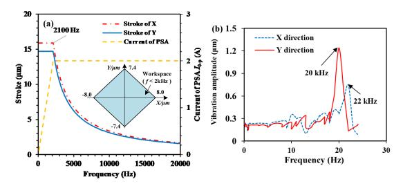
Fig. 3 Performance evaluation of second-generation tool. (a) stroke vs frequency. (b) dynamic tests results
