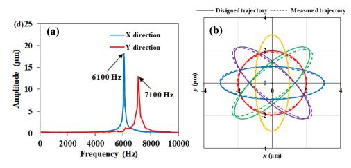
Fig. 2 Performance evaluation of first-generation tool. (a) dynamic tests results, (b) controllability of elliptical vibration trajectory
