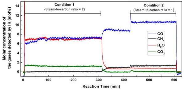
Figure 2 Molar concentrations of the important effluent gases as a function of reaction time during SMR operations measured by IR spectrometer. Note that between 0 - 430 minutes, the effluent is diluted by extra N<sub>2</sub> gas.
