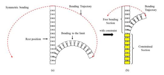
Fig. 1 Work principle of the CTSM: (a) bending of the conventional TSM; (b) in the CTSM the constraint changes the length of the bending section.
