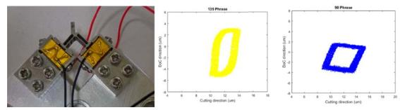
Figure 3. Prototype of non-resonant vibration cutting tool and generated arbitrary tool paths.
