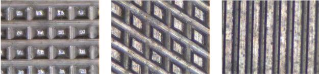
Figure 5. Machined patterned surfaces on aluminum workpieces.
