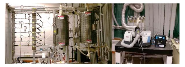
**Figure 1** The catalyst testing system. Left: reactor, gas manifold and steam generator; right: IR spectrometer with 2-m gas cell for gas detection and quantification.
