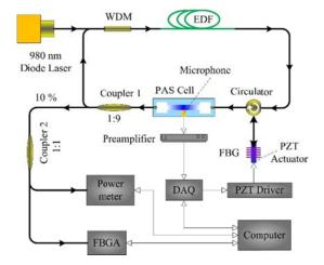
**Fig. 3.** Configuration of the FLI-PAS gas detection system. WDM, wavelength division multiplex; EDF, erbium doped fiber; FBG, fiber Bragg grating; PZT, piezoelectric transducer; DAQ, data acquisition card; FBGA, FBG interrogation analyzer.
