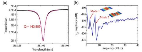
Fig. 8. (a) Optical transmission spectrum of the ring cavity showing the optical quality factor of  $1.4 \times 10^5$ . (b) Spectrum of S<sub>21</sub> magnitude collected from the vector network analyzer. The identified two peaks correspond to the fundamental ( $f_1 = 2.5$  MHz) and second-order ( $f_2 = 8.85$  MHz) mechanical modes. Their mechanical quality factors are ~10 as measured in ambient air.
