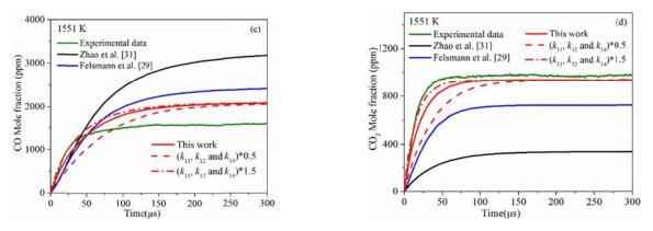
Fig. 4. Comparisons of the measured (olive line) and simulated concentration time-histories of CO and  $CO_2$  at 1369 and 1551 K and at 1.6 atm during the pyrolysis of 0.2% MP/Ar.
