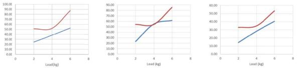
*Fig. 4. Summary of human experiments. Load vs EMG reading without robot (red) and with robot (blue). Anterior for flexion motion (left), middle for abduction (middle) and posterior for extension (right).*
