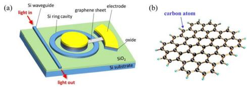
Fig. 2. (a) Optomechanical device based on hybrid integration of a Si ring cavity and a graphene nanomechanical resonator. (b) Atomic arrangement of a graphene nanosheet.
