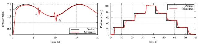
Fig. 4 (left) Trajectory tracking of the pressure controller. (right) Position regulation of the biopsy needle
