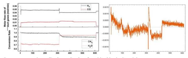
when we can experimentally observed carbon deposition kinetics in real time. **Figure 3** Catalytic performance of a 10%Ni/Al<sub>2</sub>O<sub>3</sub> catalyst in the steam reforming reactions shown in Fig. 2. Left top: H<sub>2</sub> and CO production rates; left bottom: CH<sub>4</sub> and H<sub>2</sub>O conversion rates; and right: carbon deposition rate.
