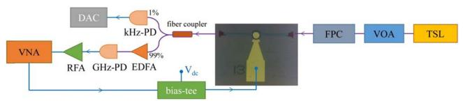
Fig. 7. Device measurement setup. VNA: vector network analyzer; RFA: radio-frequency amplifier; PD: photodetector; EDFA: erbium-doped fiber amplifier; DAC: data acquisition card; FPC: fiber polarization controller; VOA: variable optical attenuator; TSL: tunable semiconductor laser. Purple and blue wires indicate optical and electrical paths, respectively.
