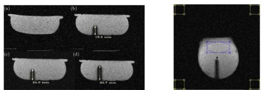
Fig. 6 (left) MRIs of the needle insertion. (right) MRI used for computing SNR of the robot
