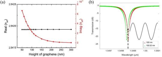
Fig. 4. (a) Real and imaginary parts of the effective index  $n_{\text{eff}}$  as a function of height of the graphene suspended above the waveguide. (b) Device's optical transmission spectra showing the result of optomechanical transduction of graphene's mechanical motion (height variation) into the optical domain.
