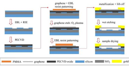
Fig. 5. Flow chart of device fabrication. EBL: electron-beam lithography; RIE: reactive ion etching; PECVD: plasma-enhanced chemical vapor deposition.
