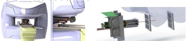
Fig. 1. (left) Conceptual MRI-guided biopsy set-up. (right) Needle insertion using the grid method
