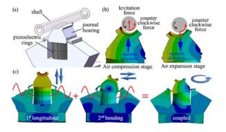
Figure 1. (a) Design of a single driving unit; (b) operation principle for shaft levitation and rotation; and (c) coupled mode shapes.
