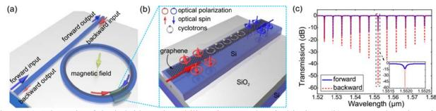
Fig. 9. (a) Schematic of the hybrid graphene/silicon integrated optical isolator. (b) A zoomed section of the isolator showing mechanism of the nonreciprocal optical transmission. (c) Calculated forward and backward light transmission spectra of the proposed device.
