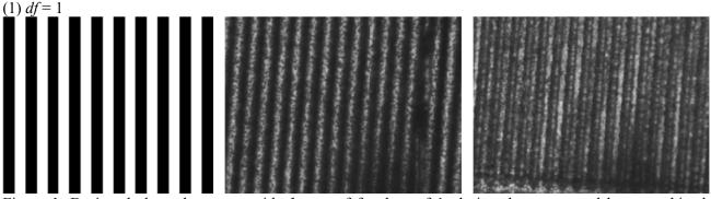
Figure 1. Designed channel patterns with degree of freedom of 1: designed patterns and laser machined patterns.
