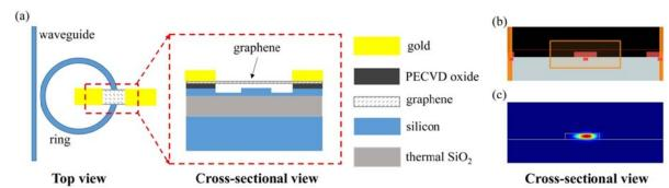
Fig. 3. (a) Top and cross-sectional views of the hybrid integrated graphene/silicon nano-optomechanical resonator. (b) Structure of the model in Lumerical mode solution. (c) Simulated optical mode profile
