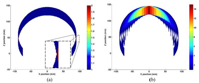
Fig. 4 Dexterity comparison of the WFM and CTSM: (a) dexterity distribution of the WFM; (b) dexterity distribution of the CTSM.
