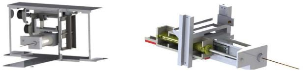
Fig. 2 (left) Conceptual model of the 3-DOF robot. (right) Details of the insertion mechanism
