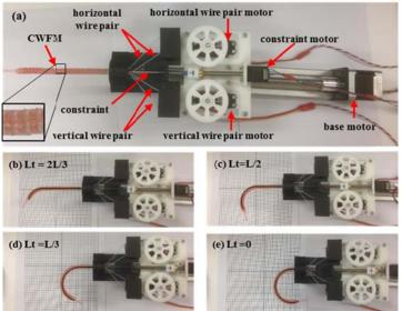
Fig.6 Proof of concept robot prototype based on the CTSM.
