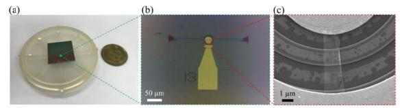
Fig. 6. (a) Device chip in sample box along with a Hong Kong 50-cent coin as a reference. (b) Optical microscope image of a hybrid integrated graphene/silicon nano-optomechanical device. (c) Scanning electron microscope image zooming in at the graphene nanosheet suspended above the waveguide of the ring cavity.
