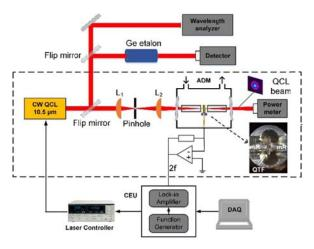
**Fig. 2.** Schematic and photo of the QEPAS sensor setup for  $C_2H_4$  detection.  $L_1$ ,  $L_2$ : plano-convex lens; ADM, acoustic detection module; QTF, quartz tuning fork; mR, micro-resonator; CEU, control electronics unit; DAQ, data acquisition.
