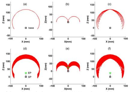
Fig. 3 Comparison of the workspace in the  $X_wZ_w$  plane: (a)-(c) workspace of the conventional wire-driven mechanism (WFM), concentric tube mechanism (CTM) and CTSM with a fixed base; (d)-(f) workspace of
