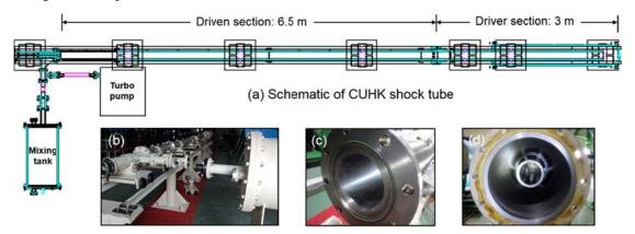
**Fig. 1.** (a) The stainless-steel, 10-m long shock tube recently built for high-temperature chemical kinetics study. (b) The polished driven section with six pairs of optical windows. (c) The driver section with an insert to achieve uniform shock conditions.
