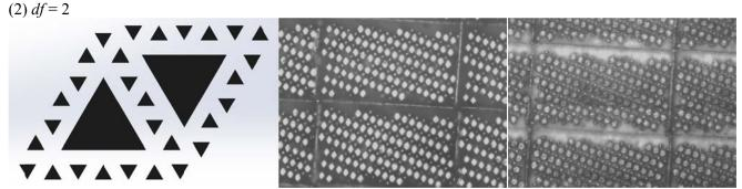
Figure 2. Designed diamond patterns with degree of freedom of 2: designed patterns and laser machined patterns.
