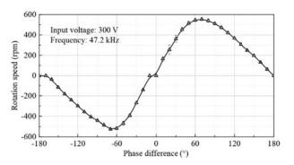
Figure 2. The relationship between rotation speed and phase angle.
