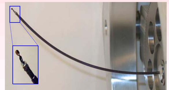
1 mm wide MEMS forceps mounted on a needle-like robot arm.
