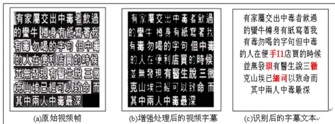
Figure 3. Illustration of the process of video caption recognition – (a) shows the original extracted captions from a video frame, (b) shows the enhanced captions and (c) shows the recognition outputs.
