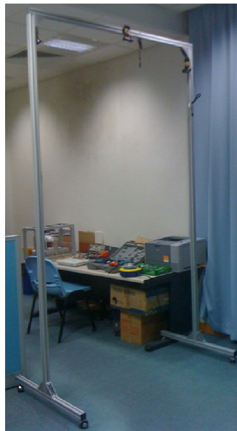
Figure 12. A new setup to capture the full human body shape by cameras.
