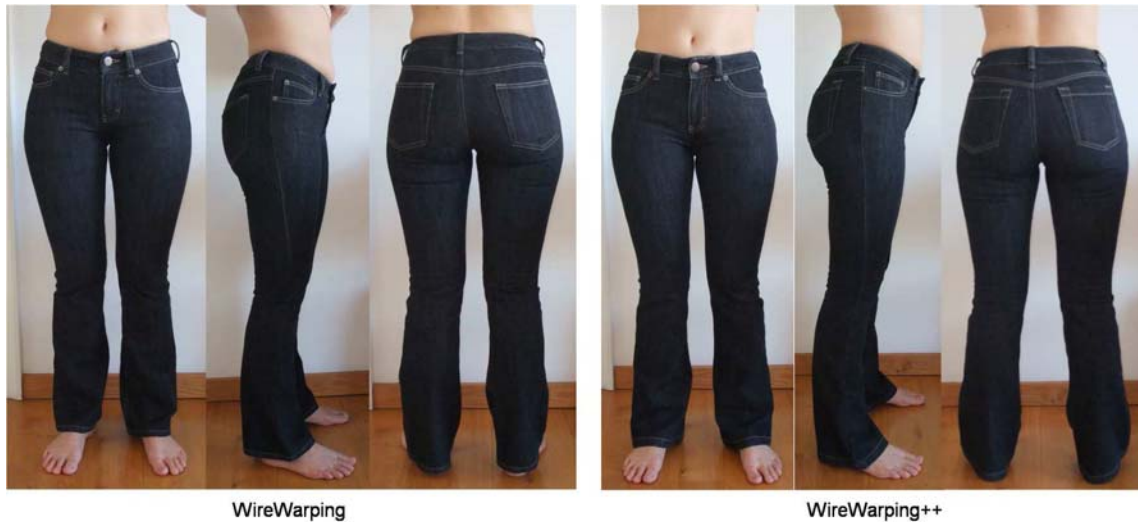
Figure 6. Photos of the jeans pants fabricated from the patterns generated by WireWarping versus those generated by WireWarping++. The one generated by WireWarping++ fits the back waist band and the back yoke much better – this is the comment made by a fashion specialist.
