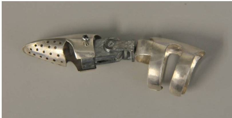
Figure 5. A non-invasive ring like structure for attachment
