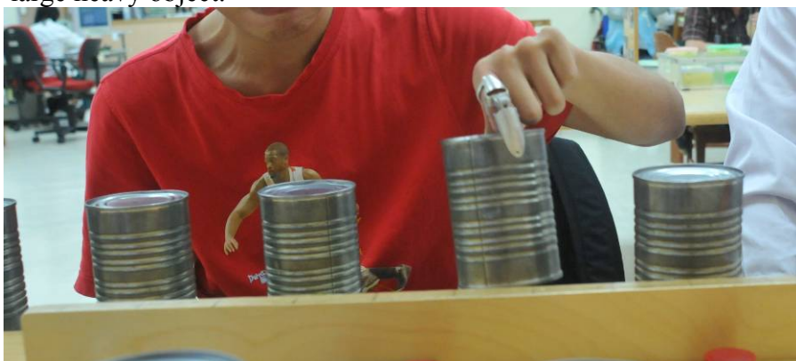
Figure 8. Pick up a heavy object with the help of prosthesis
