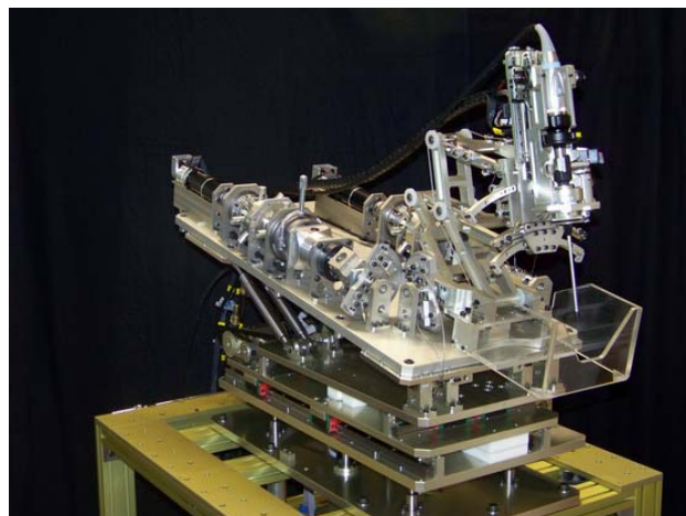
Fig. 2 The developed robotic endoscope holder.
