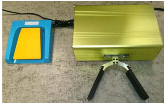
Fig. 4 The foot-controlled interface.
