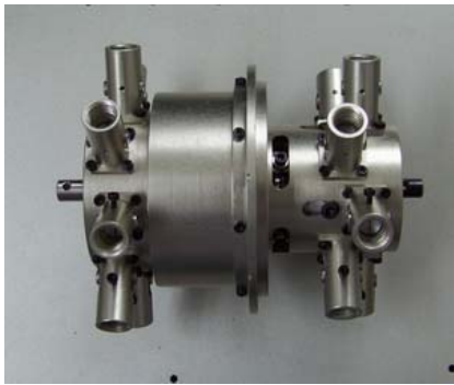
Fig. 3 The passive safety protection mechanism installed at the joints.
